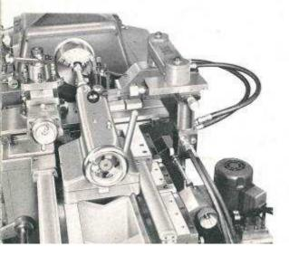
The wide range of attachments available for use on this lathe includes thread chasing, taper turning, spherical turning, grinding and hydraulic profiling equipment (illustrated). Spindle speed reduction units and various types of toolbox are also available.
